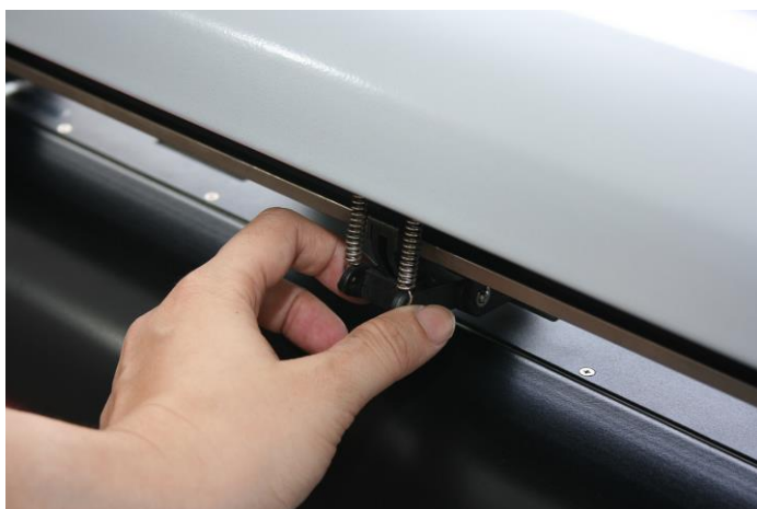
Figure 4-3 correct way to move pinch rollers
